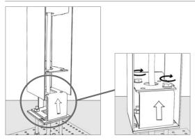
Insert the device body on the bracket and lock the bolts using a CH5 10Nm key
