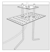
Cement the anchor bolt flush by passing the cable through the appropriate openings
