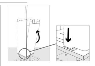
Slide the cover into the spaces provided on the device surface
