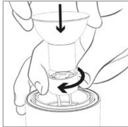
Insert bulb MR11 into GU4 lamp holder, using internal bulb support
