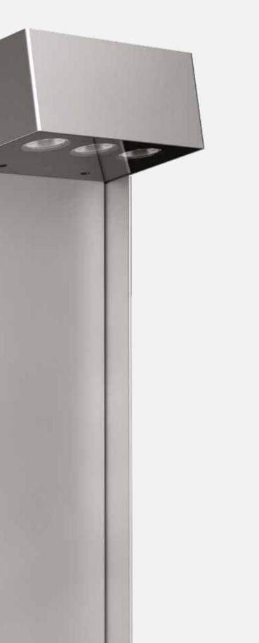
Bollard available in a single height of 19.7", made of AISI 316L stainless steel. Pole head with 3 LEDs and 65° optic. Available in 2700K, 3000K and 4000K versions. Flush black silk-screened glass, extra-clear tempered 0.16" thick. Integrated power supply. Flange with anchor bolts for installation in concrete. HCT surface finish available in three variants.
