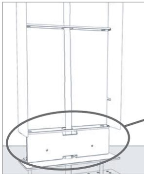
Insert the device body on the bracket and lock the bolts using a CH5 10Nm key
