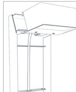
Insert the device body and lock using Torx T9 key for upper screws and Allen key size 2.5mm for lower screws
