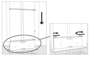
Insert the device body on the bracket and lock the bolts using a CH5 10Nm key
