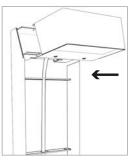
Insert the device body and lock using Torx T9 key for upper screws and Allen key size 2.5mm for lower screws
