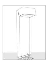
Slide the cover into the spaces provided behind the device and lock using an allen key
