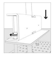
Insert the bracket and lock the bolts with a CH10 10Nm key
