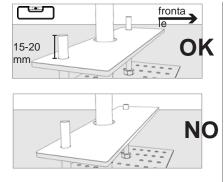
Check that everything is perpendicular to the bubble level of the surface, an incorrect positio-ning will cause the device to become unstable
