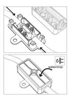
Cable wiring using waterstop connector Suggested cable cross-section - up to 2 x 18 AWG. Cable External diameter min. - max. 0.189" - 0.236" DIA.
