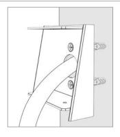
Fix the bracket by guiding the cable through the cable slot
