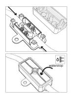
Cable wiring using waterstop connector Suggested cable cross-section - up to 2 x 18 AWG. Cable External diameter min. - max. 0.189" - 0.236" DIA.
