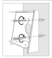
Drill the wall in the traced marks, insert the fixing plugs and align the bracket and screws
