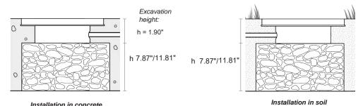
Leave under the casing 7.87"/11.81" of drainage material (do not use sand that can be compacted) praper drainage and avoid stagnant water
