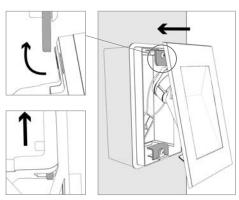
Incline the luminaire to be able to insert the upper part correctly into the casing, Finally press it down until it its
