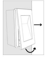
Leverage the bottom of the frame to unlock and remove the device from the casing
