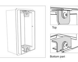
Pay attention to the positioning direction of the casing in order to properly install the device
