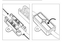
Cable wiring using supplied water stop connector
