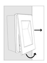
Leverage the bottom of the frame to unlock and remove the device from the casing
