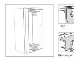
Pay attention to the positioning direction of the casing in order to properly install the device
