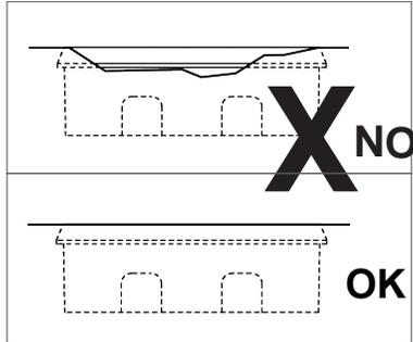
Install the casing on a flat floor
