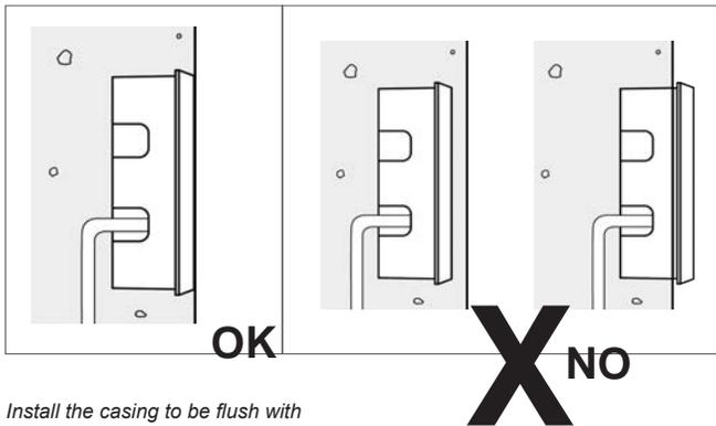
Install the casing to be flush with the wall
