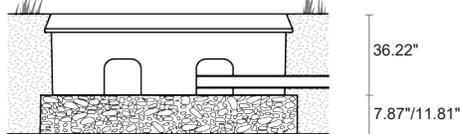
Leave under the casing 7.87"/11.81" of drainage material (do not use sand that can be compacted) proper drainage and avoid stagnant water.
