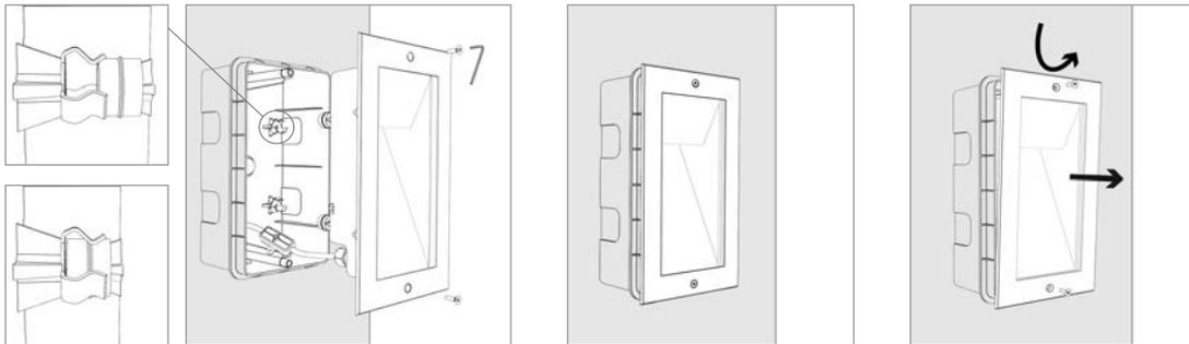
Align and insert the device into the casing, press down until interlocking, and then tighten the screws using a 2 mm Allen screw
