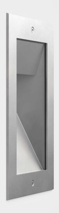
Frame and body made of AISI 316L stainless steel. Optical reflector in AISI 316L stainless steel for grazing lighting. Applied tempered shielding glass 0.16" thick. Wide and symmetrical optics at 2700K, 3000K and 4000K. Stainless steel fixing screws with color matched to the finish. Wall installation with polyethylene outer casing. Integrated power supply. HCT surface finish available in three variants.
