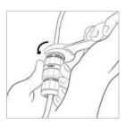
Fasten cables to the connector
