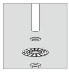
Screw the first nut into the lower part of the an-chor bolt, insert the fixing plate and secure with the counter nut. Flush the anchor bolt by feeding the cable through the anchor bolt tube.
