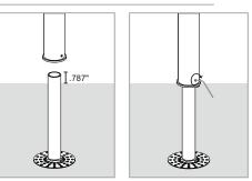
Screw the pole to the anchor bolt and secure with the grub screw
