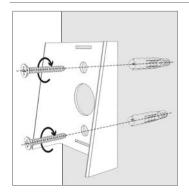
Drill the wall in the traced marks, insert the fixing plugs and align the bracket and screws
