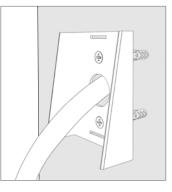
Fix the bracket by guiding the cable through the cable slot
