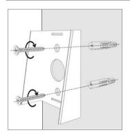
Drill the wall in the traced marks, insert the fixing plugs and align the bracket and screws
