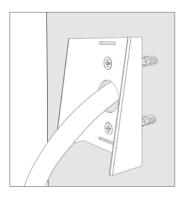
Fix the bracket by guiding the cable through the cable slot
