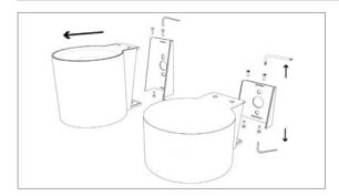
Disassemble device body using T9 Torx key for upper screws and 2.5 mm Allen key for lower screws
