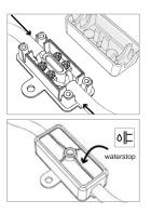
Cable wiring using waterstop connector
