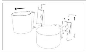
Disassemble device body using T9 Torx key for upper screws and 2.5 mm Allen key for lower screws For bi-directional version, use the Allen key for both screws
