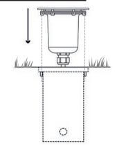
Aligning and installing the device in the casing
