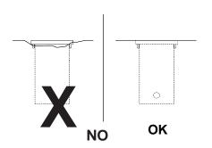
Install the casing on a flat floor
