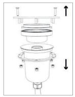
Disassemble device body using 2.5 mm Allen screw and 7 mm hex key
