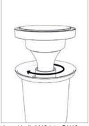
Insert bulb M16 into GU10 lamp holder, using internal bulb support
