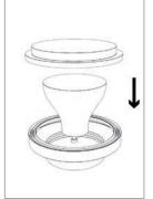
Insert the MR16 lamp into the gasket and then reinsert
