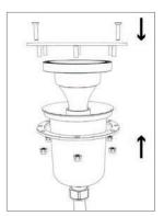
Reassemble device body by screwing through 2.5 mm Allen screw and 7 mm hex key
