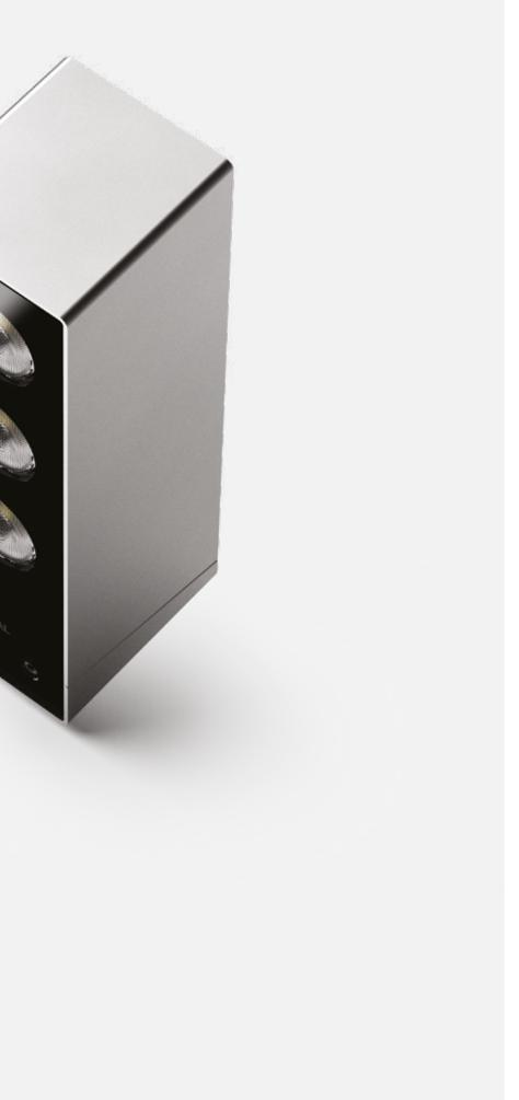
The spacer integrated with the lamp body makes the product compact. Bracket with joint for 360° rotation on one axis. Made of AISI 316L stainless steel. Flush black silk-screened glass extra-clear tempered, 0.16" thick. Single-emission version with one, two or three LEDs for different design needs. 21°, 45° and 65° optics at 2700K, 3000K and 4000K. Integrated power supply. HCT surface finish available in three variants.
