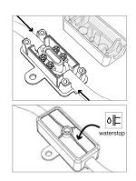
Cable wiring using water stop connector
