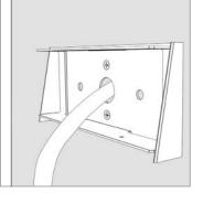
Fix the bracket by guiding the cable through the cable slot
