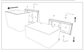
Disassemble device body using T9 Torx key for upper screws and 2.5 mm Allen key for lower screws
