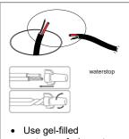
Use gel-filled waterproof wire-nuts for wire connections.  It is the contractor's responsibility to install Remote Driver in a suitable electrical enclosure.
