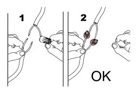
Use gel-filled waterproof wire-nuts for wire connections.
