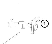
Drill into the wall to insert predisposed lamp elements
