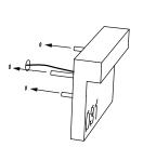
Fix the body lamp in the holes wall with glue, making sure not to press the cable.
