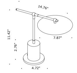
R50.021 LED single 1W Rechargeable battery provided with 120VAC charger DIM. 2700K 140 lm IP44
