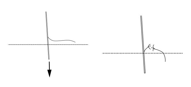
Insert the copper stem into the ground until the cable is flush with the ground
