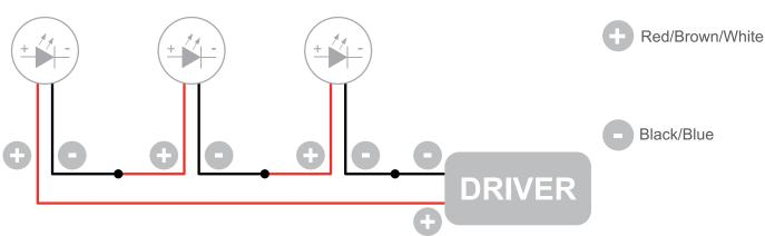
The individual lamps must be connected in series.
