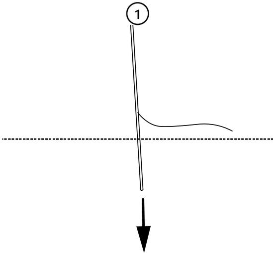
Insert the copper stem into the ground until the cable is flush with the ground
