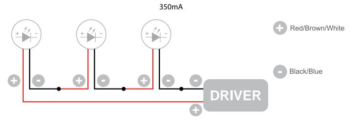
The individual lamps must be connected in series.
