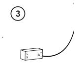
Connect the remote driver with 120VAC power supply, LED input respecting +/- polarity
