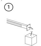
Create a concrete basement with central light point and connect the cable coming out of the pole with the ground light point respecting the polarity (+/-) using waterproof wire-nut
