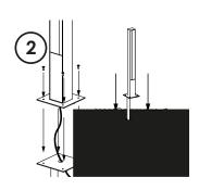
Fix the lamp body on the picket using the screws and insert it in the ground
