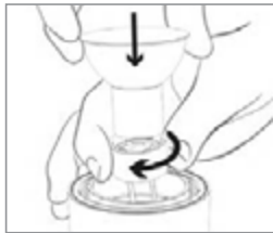
Insert bulb M11 into GU4 lamp holder
