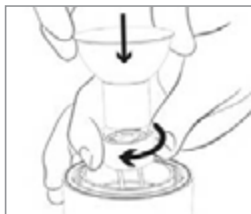
Insert bulb M11 into GU4 lamp holder
