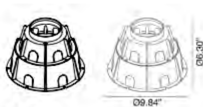
PT52122 Casing for ground recessing 9.84" x 6.30"
