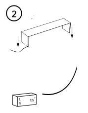
Place the bench in desired position connect the remote power supply respecting the 12V output, polarity +/- and 120VAC mains input
