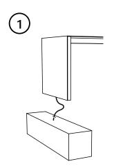
Create a concrete a base with central light point and connect the the low voltage ground light point with the cable of the seat respecting the polarity +/-
