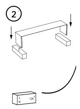
Place the bench on the base connect the remote power supply respecting the 24V output, polarity +/- and 120VAC mains input
