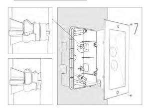
Align and insert the device into the casing, press down until interlocking, and then tighten the screws using a 0.08" Allen screw
