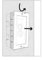
Remove the screws using a 0.08" Allen screw, pry the back of the frame to unlock and remove the device from the casing
