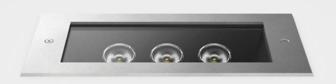
Frame and lamp body in stainless steel, including the part recessed in the ground. Stainless steel fixing screws with color matched to the finish. Horizontal or vertical asymmetrical reflector. Optics from 21°, 45° and 65° at 2700K, 3000K and 4000K. Installation in the ground and/or on the floor through polyethylene outer casing. 0.31" (8mm) extra-clear tempered glass. Integrated power supply. HCT surface finish available in three variants.
