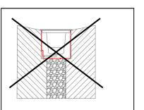
Note: Never install the fixtures in the ground with wrong incline because this could be the cause of dirty deposit and permanent submersion of fixture. The parts of the fixtures are damaged owing to stagnation and aggressive chemical elements. The fixture must be protected from direct contact with the ground by the junction box in plastic material.
