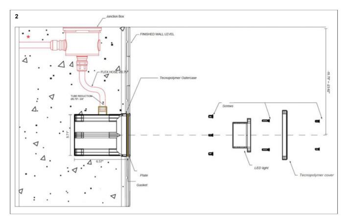
MINI DOLPHIN installation scheme for concrete with tile. Recommended mounting height -15.75" ÷ -23.62" in from the edge of the water
