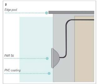
Install in concrete pools with PVC or tile coating.
