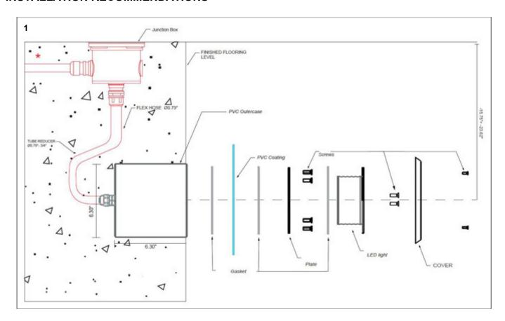
SQUID installation scheme for PVC coating.
