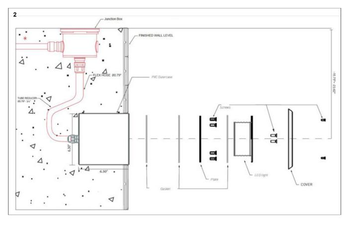
SQUID installation scheme for concrete with tile. Recommended mounting height -15.75" ÷ -23.62" in from the edge of the water
