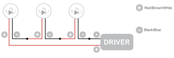
The individual lamps must be connected in series. Only power up the system once all the lamps have been connected.
