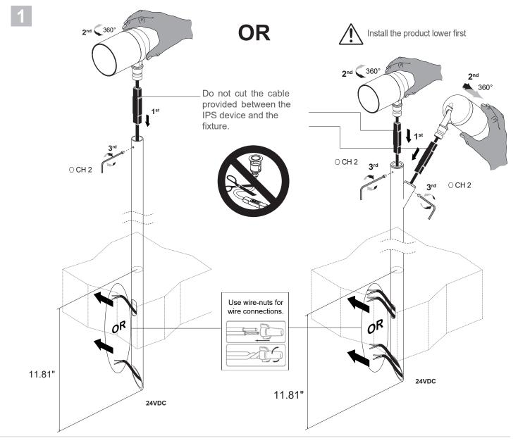
• It is the contractor's responsibility to caulk around the edges between the fixture and the mounting surface, to satisfy wet label requirements.
