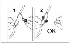
Make proper wiring connections and slide through the middle hole in the back of the base and through the mounting base assembly as shown.
