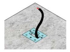
INSERT THE BASE & LET THE WIRE THROUGH ITS BOOTTOM CLEARANCE HOLE
