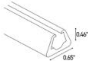
OUT-S-9.5x6.5.F/W White Flexible Silicone Outercase L=16.40'
