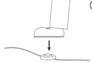
Push the foot dimmer button to switch on the lamp
