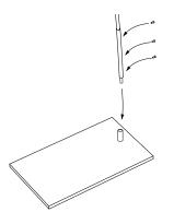
Insert the rod into the hole of the plate, tighten the screws for locking
