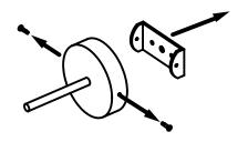
1. Disassemble the bracket and fix it to the wall.
