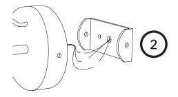
Complete the wiring with 120V power supply. Connect the yellow/green ground wire
