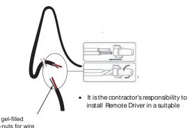
Use gel-filled wire-nuts for wire connections.
