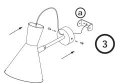
Fix the structure to brackets 'a' and screw the bulb into the lamp
