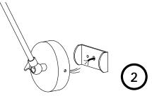
Complete the wiring with 120V power supply. Connect the yellow/green ground wire
