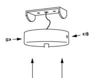
${\bf 3.Fix}$  the structure to the bracket, tighten the side screws, and screw the glass
