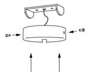
3. Fix the structure to the bracket, tighten the side screws, and screw the glass
