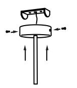
3. Fix the structure to the bracket
