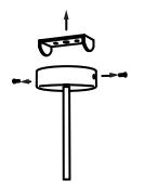
1. Undo the screws and fix the bracket to the ceiling
