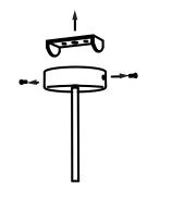
1. Undo the screws and fix the bracket to the ceiling
